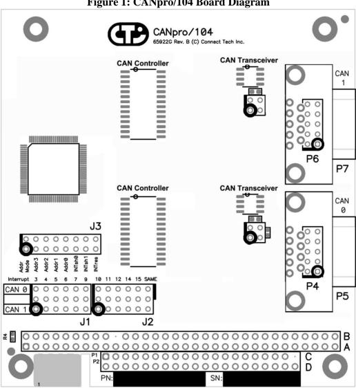
Figure 1: CANpro/104 Board Diagram
